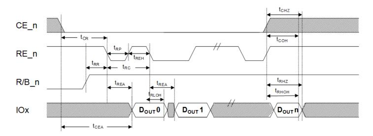
Figure 4-28 EDO data output cycle timings
