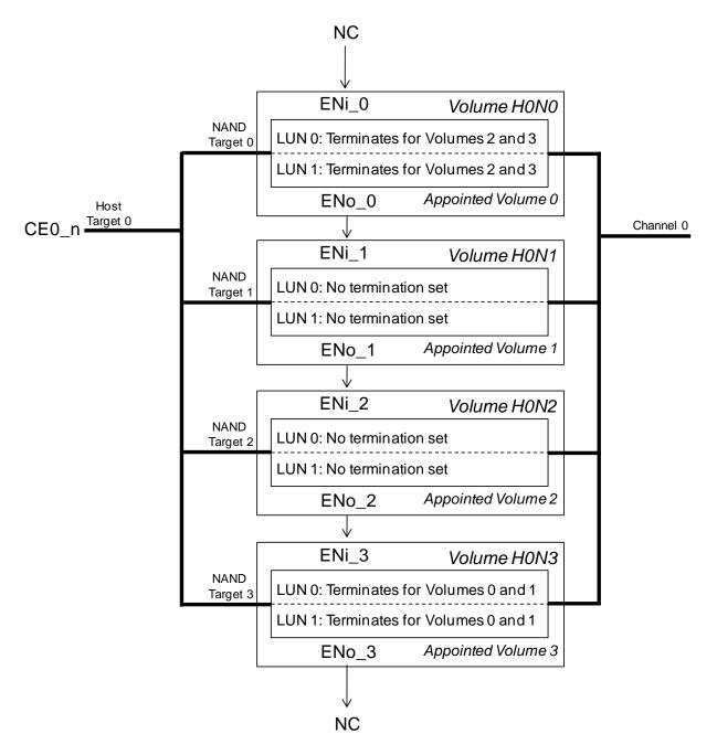
Figure 4-21 Example: Parallel Non-Target ODT
