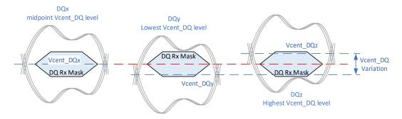
Figure 4-23 NV-DDR3/NV-LPDDR4 Vcent\_DQ (pin\_mid) Definition
