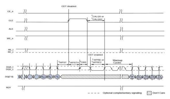
Figure 4-1 Example of Data Input Burst Exit with CLE=1 and Resume with CLE=0
