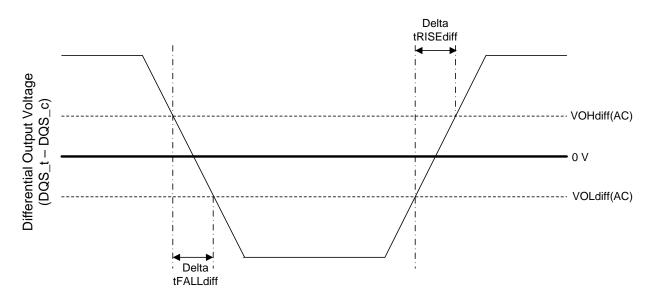
Figure 4-9 tRISEdiff and tFALLdiff Definition for Output Slew Rate, NV-DDR2/3, NV-LPDDR4 (differential)
