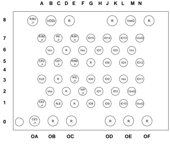
Figure 2-4 LGA pinout for 16-bit data access
