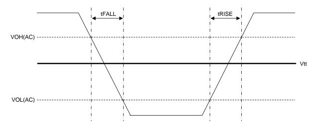
Figure 4-8 tRISE and tFALL Definition for Output Slew Rate, NV-DDR2/3, NV-LPDDR4 (single-ended)
