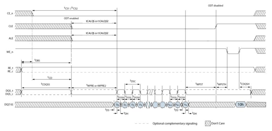
Figure 4-42 Data input cycle timing
