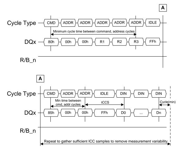
Figure 7-5 ICC4W measurement procedure
