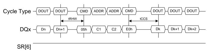
Figure 5-34 Change Read Column timing
