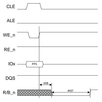
Figure 5-5 Reset timing diagram
