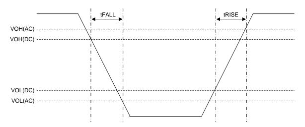
Figure 4-7 tRISE and tFALL Definition for Output Slew Rate, NV-DDR
