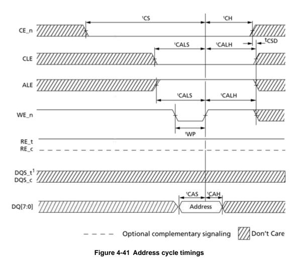
NOTE: When the bus state is not a data input or data output cycle, if ALE, CLE and CE\_n are all low (i.e. Idle state) then DQS (DQS\_t) shall be held high by the host to prevent the device from enabling ODT. If ODT is disabled, then DQS is a don't care during Idle states.
