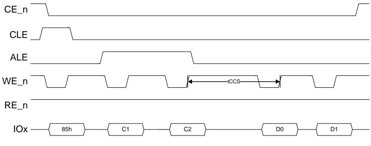
Figure 5-2 SDR data interface command description
