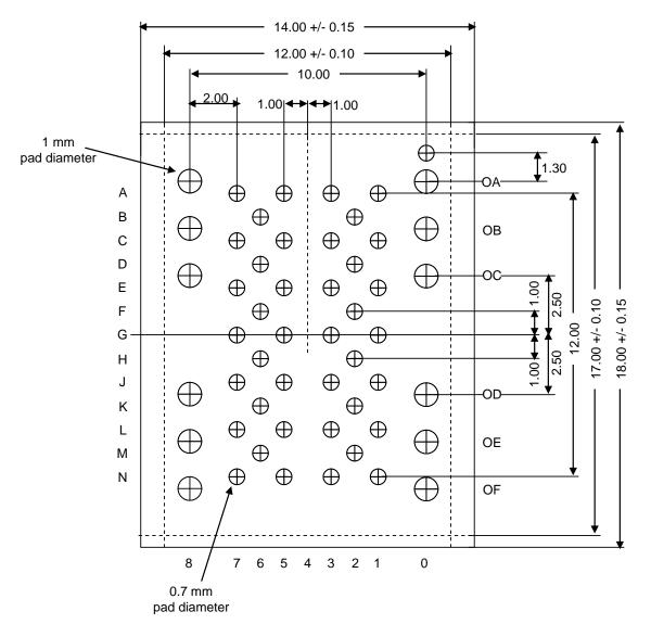
Figure 2-5 LGA-52 pad spacing requirements (bottom view, dimensions in millimeters)
