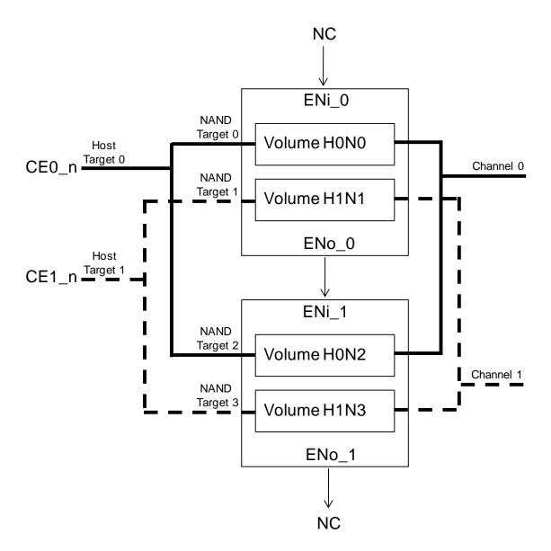
Figure 2-35 CE\_n Pin Reduction Topology, example 2
