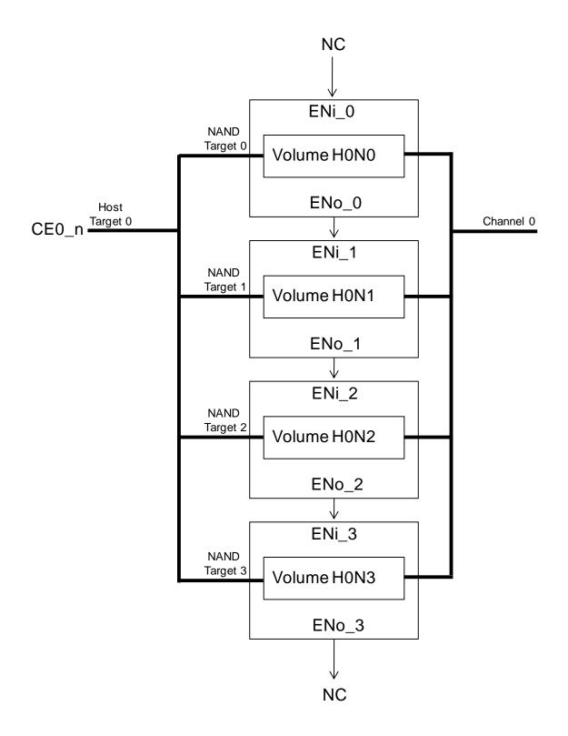
Figure 2-34 CE\_n Pin Reduction Topology, example 1
