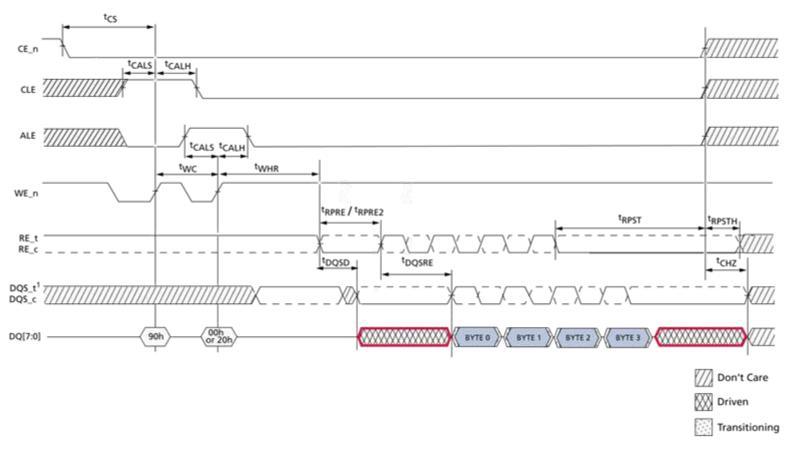
Figure 5-12 Read ID command using NV-DDR2 NV-DDR3 or NV-LPDDR4 data interface
