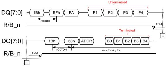
Figure 5-41 ODT Disable/Enable Timing
