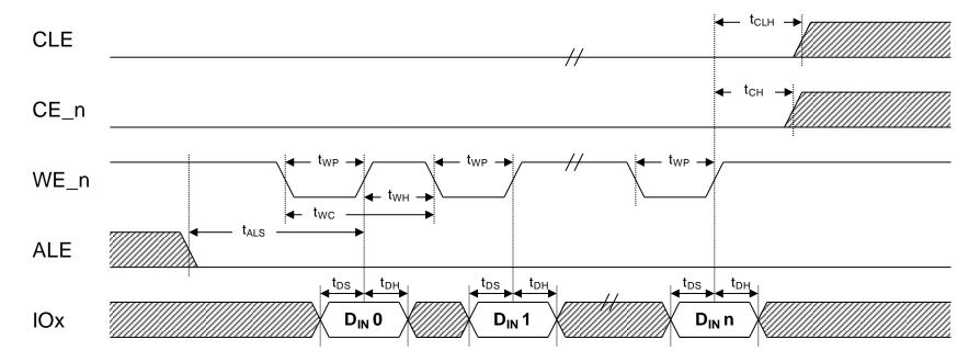
Figure 4-26 Data input cycle timings
