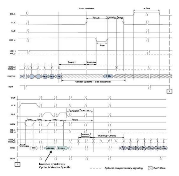
Figure 4-3 Example of Data Input Burst Exit with CE\_n High > 1uS and Resume Sequence for Devices that support greater than 800 MT/s
