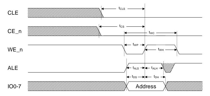
Figure 4-25 Address latch timings
