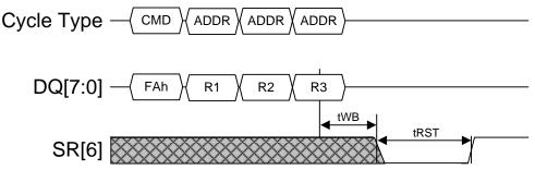
Figure 5-7 Reset LUN timing diagram
