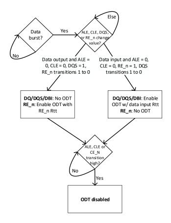
Figure 4-17 Self-termination only ODT Behavioral Flow
