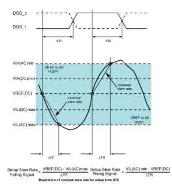
Figure 4-12 Nominal Slew Rate for Data Setup Time (tDS)
