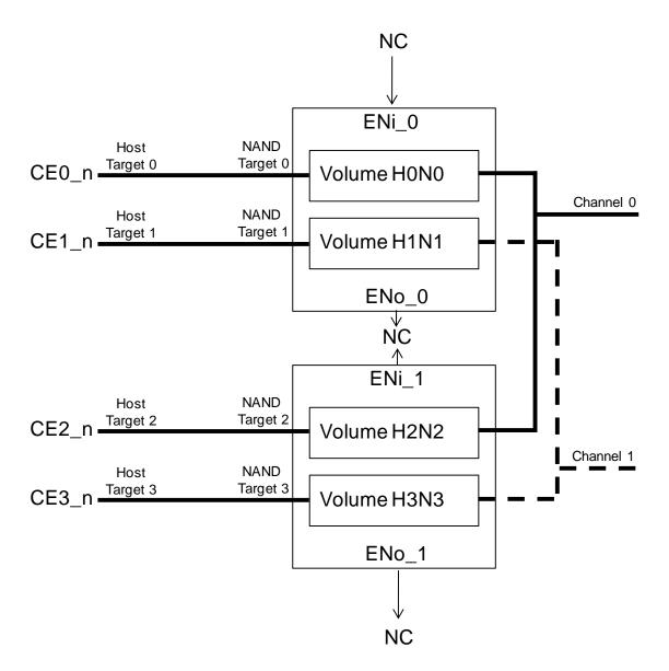
Figure 2-36 Discrete CE\_n per package topology
