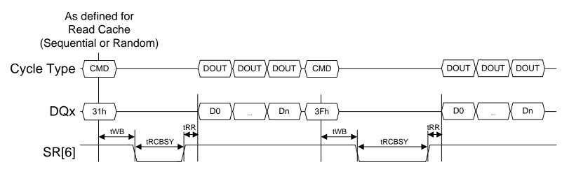
Figure 5-24 Read Cache timing, end of cache operations
