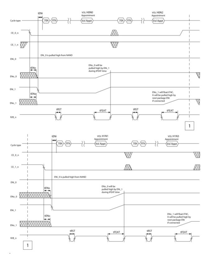
Figure 3-7 Example of Sequential Reset Initialization of Figure 2-35 Topology
