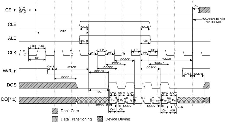
Figure 4-36 Data output cycle timing
