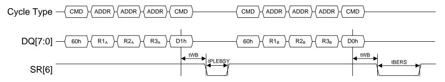
Figure 6-8 Multi-plane Block Erase timing
