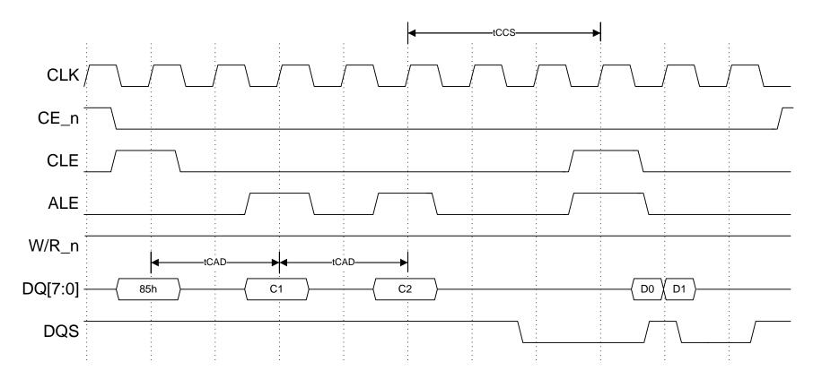
Figure 5-3 NV-DDR data interface command description
