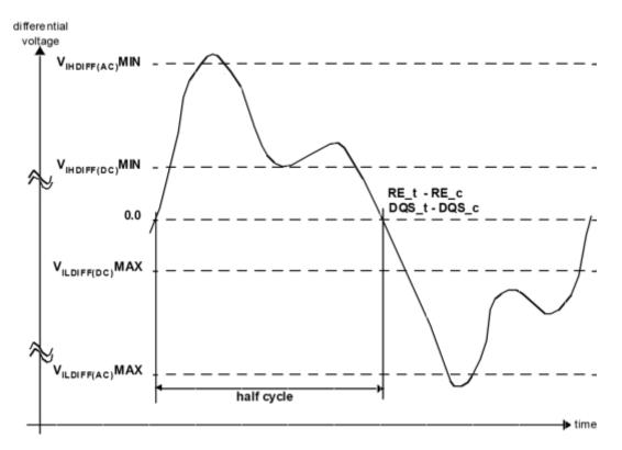
Figure 2-29 Definition of Differential AC Swing
