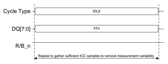
Figure 7-6 ICC5 measurement procedure
