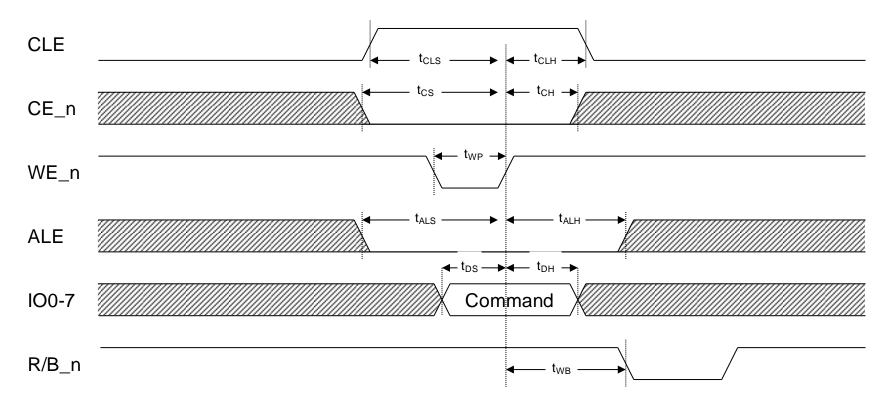
Figure 4-24 Command latch timings
