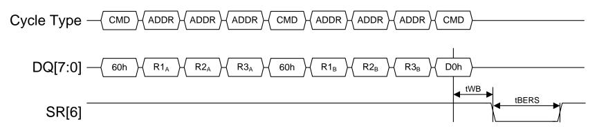
Figure 6-9 Multi-plane Block Erase timing, ONFI-JEDEC Joint Taskgroup primary definition
