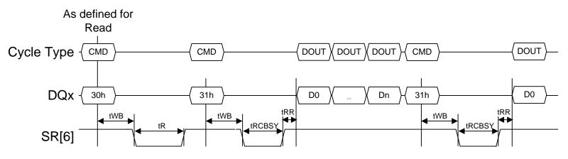
Figure 5-22 Read Cache Sequential timing, start of cache operations
