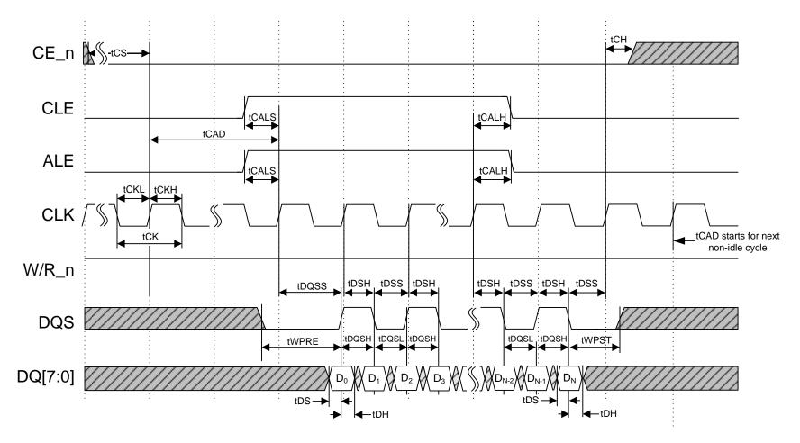
Figure 4-33 Data input cycle timing
