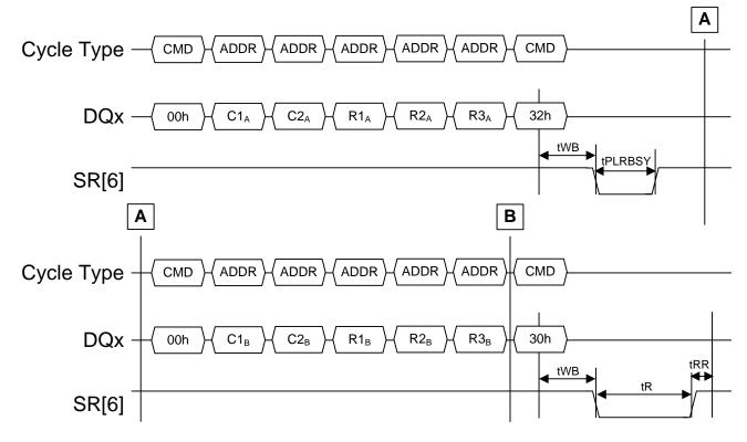
Figure 6-10 Multi-plane Read command issue timing
