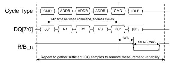
Figure 7-3 ICC3 measurement procedure
