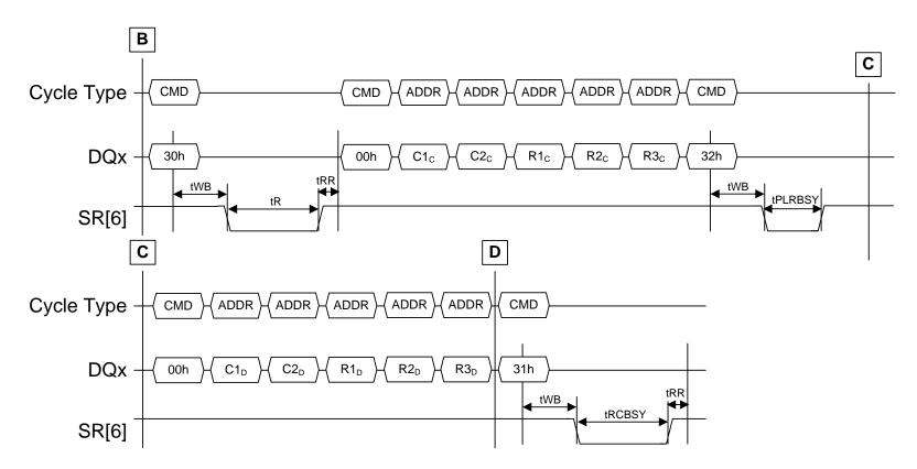
Figure 6-13 Multi-plane Read Cache Random command issue timing
