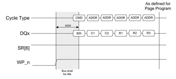
Figure 2-33 Write Protect timing requirements, example
