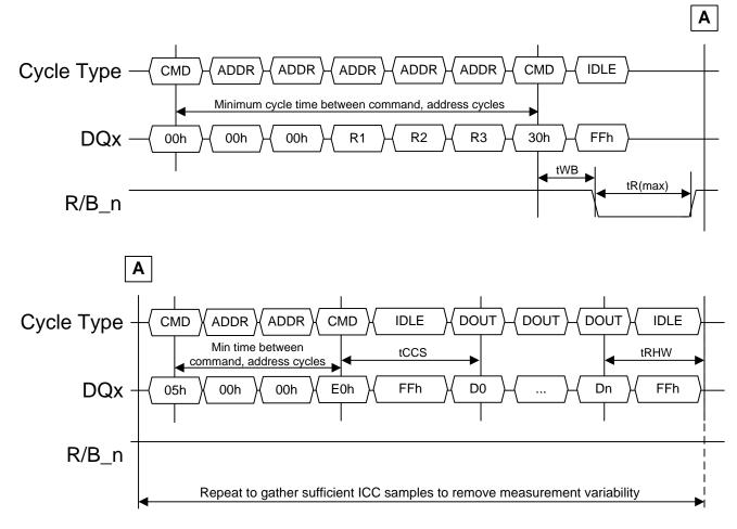
Figure 7-4 ICC4R and ICCQ4R measurement procedure
