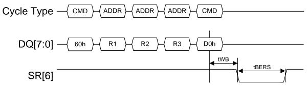
Figure 5-15 Block Erase timing
