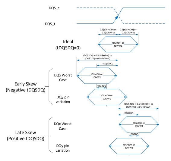
Figure 4-43 Data input cycle timing (before training)
