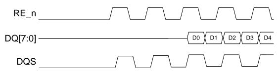
Figure 4-16 Warmup Cycles for Data Output
