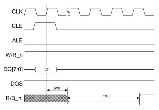
Figure 5-6 Synchronous Reset timing diagram
