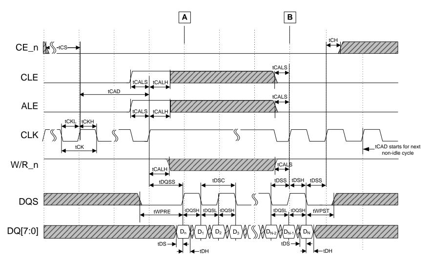
Figure 4-34 Data input cycle timing, CLK stopped
