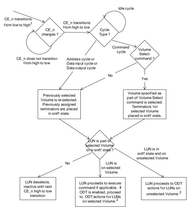
Figure 3-4 defines the Volume reversion requirements when CE\_n transitions from high to low.
