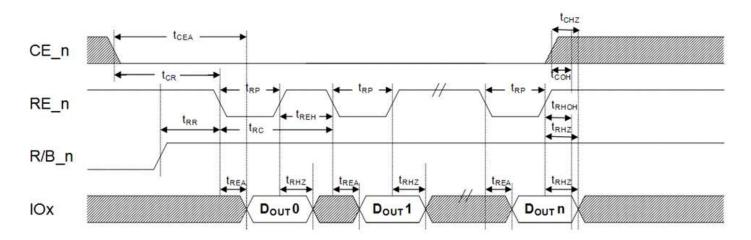
Figure 4-27 Data output cycle timings
