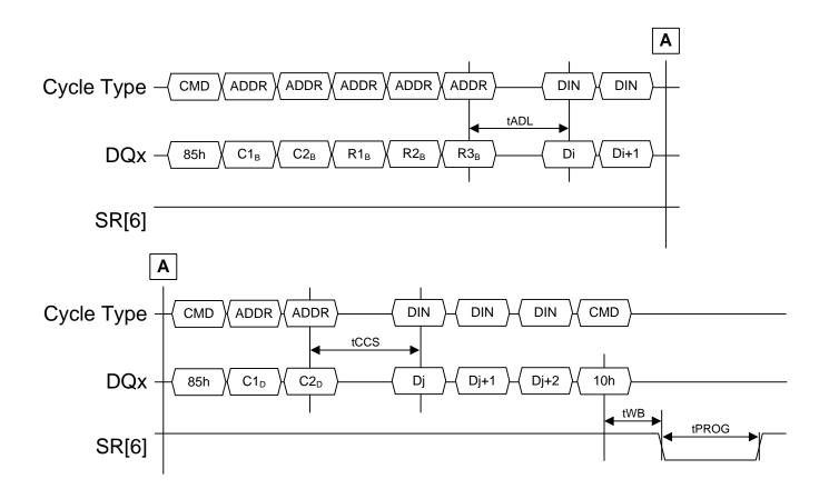
Figure 5-31 Copyback Program with data modification
