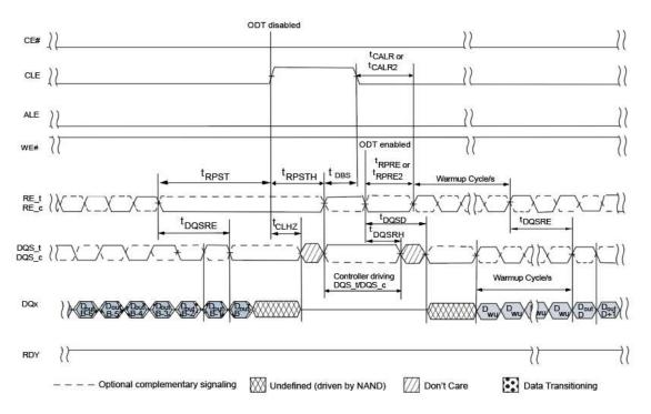
Figure 4-2 Example of Data Output Burst Exit with CLE=1 and Resume with CLE=0
