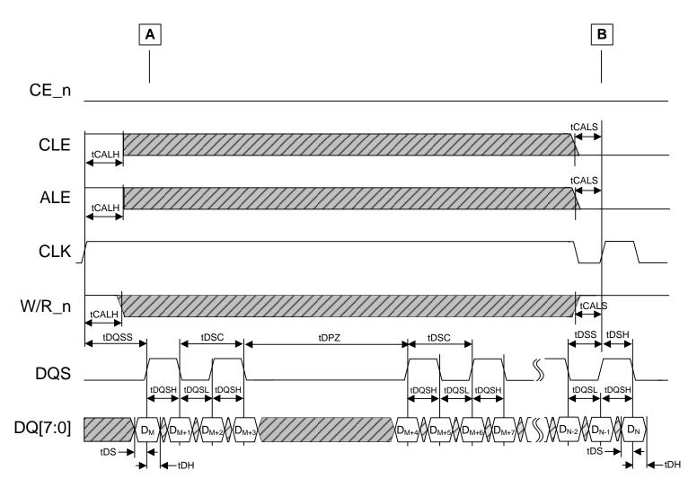
Figure 4-35 Data input cycle timing, CLK stopped with data pause
