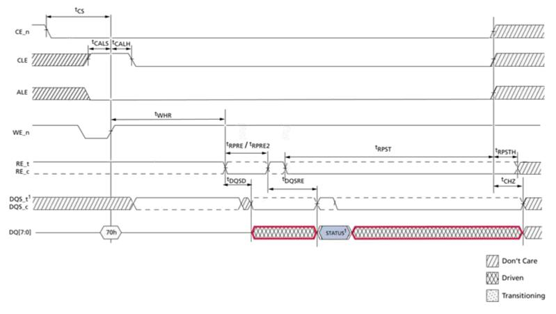
Figure 5-19 Read Status command using NV-DDR2/3 and NV-LPDDR4 data interface
