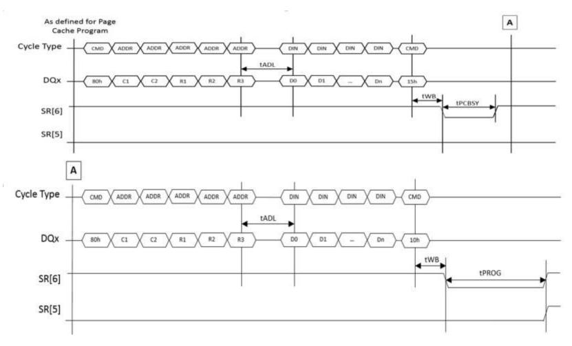
Figure 5-27 Page Cache Program timing, end of operations using 10h
