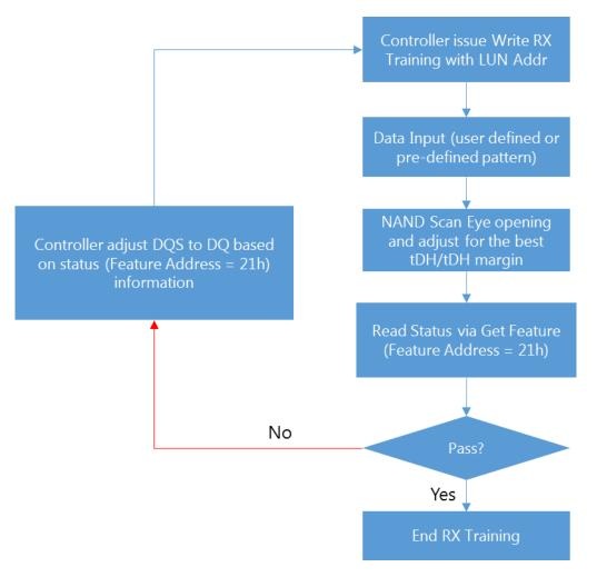
Figure 5-54 Flow chart for Write DQ Training (Rx side)
