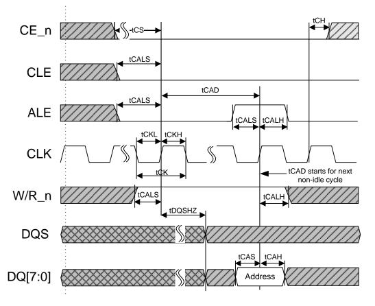
Figure 4-32 Address cycle timings
