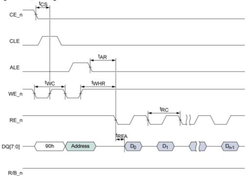
Figure 5-10 Read ID command using SDR data interface
