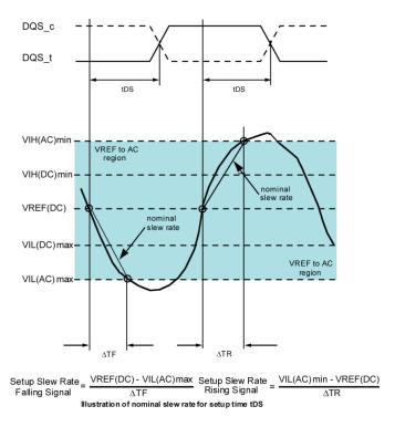
Figure 46 Nominal Slew Rate for Data Setup Time (tDS)
