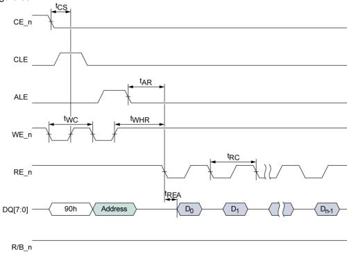
Figure 87 Read ID command using SDR data interface
