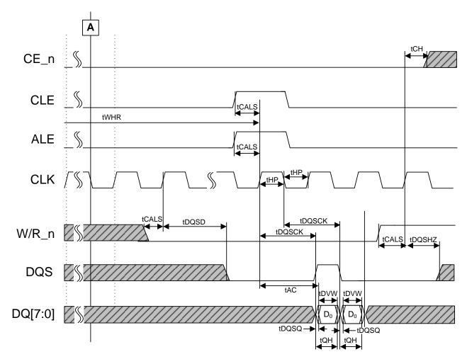
Figure 71 Read Status including tWHR and tCAD timing requirements, continued
