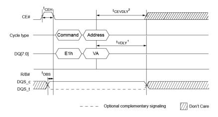
Figure 115 Volume Select timing diagram
