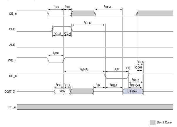
Figure 94 Read Status command using SDR data interface
