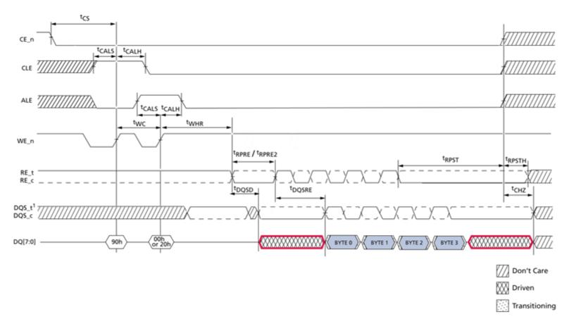
Figure 89 Read ID command using NV-DDR2 or NV-DDR3 data interface
