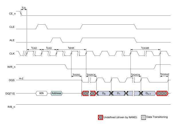
Figure 88 Read ID command using NV-DDR data interface
