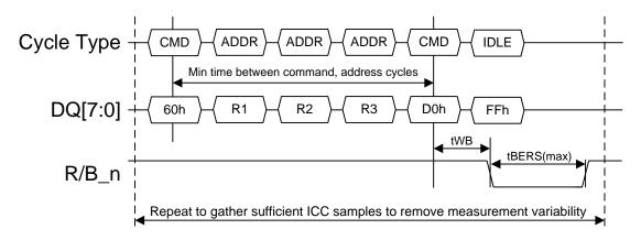
Figure 146 ICC3 measurement procedure
