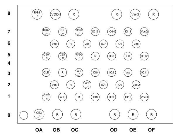
Figure 5 LGA pinout for 16-bit data access
