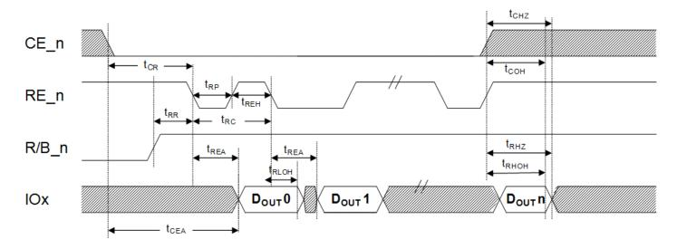
Figure 60 EDO data output cycle timings
