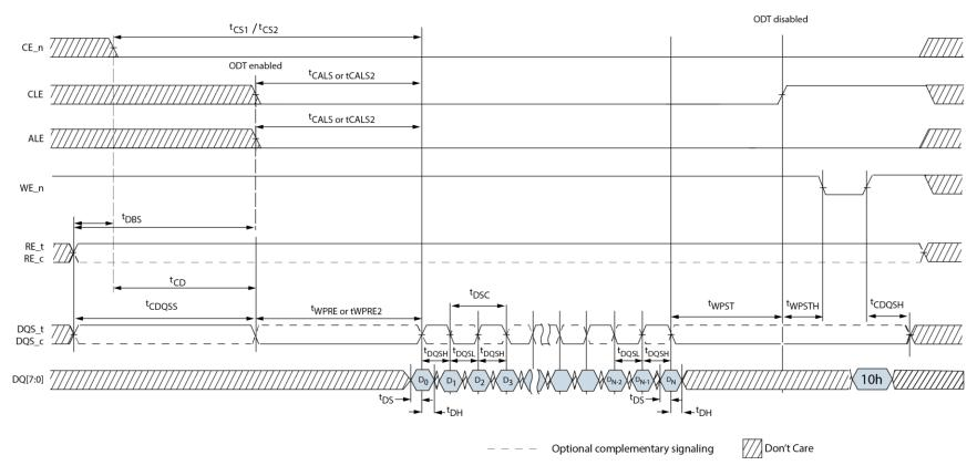
Figure 74 Data input cycle timing (no training)
