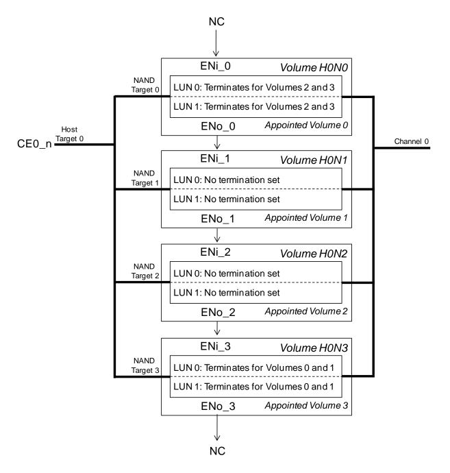
Figure 55 Example: Parallel Non-Target ODT
