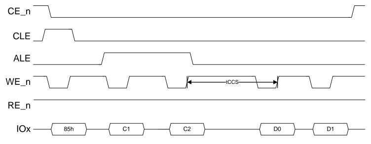
Figure 79 SDR data interface command description
