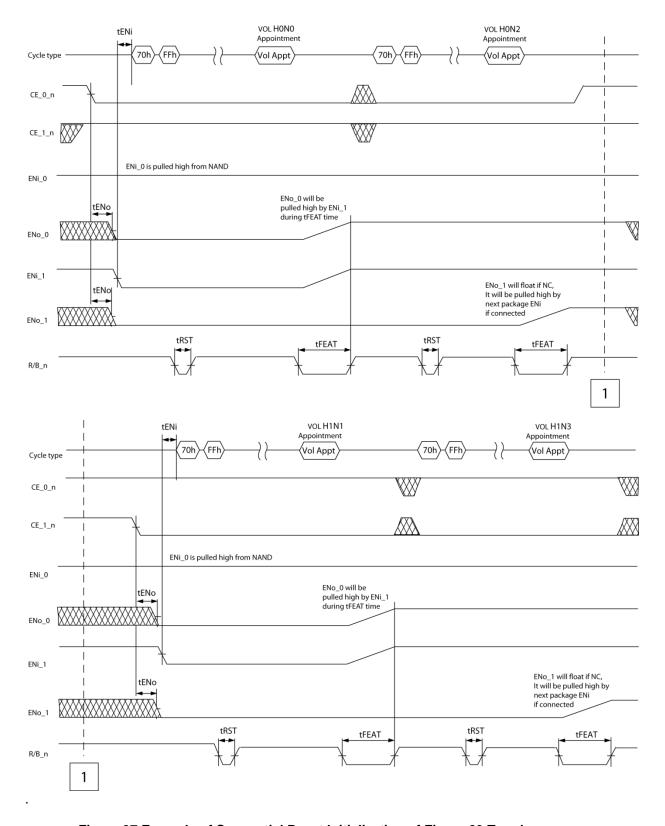
Figure 37 Example of Sequential Reset Initialization of Figure 29 Topology
