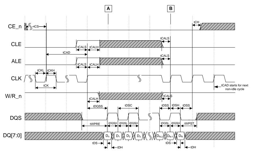
Figure 66 Data input cycle timing, CLK stopped
