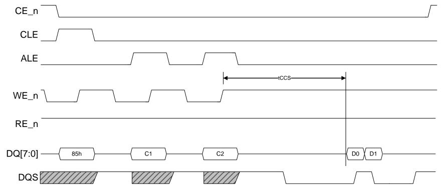
Figure 81 NV-DDR2 and NV-DDR3 data interface command description
