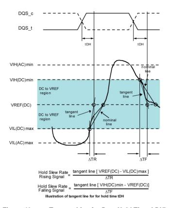
Figure 49 Tangent Line for Data Hold Time (tDH)
