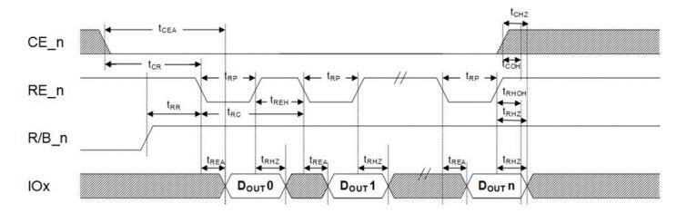
Figure 59 Data output cycle timings
