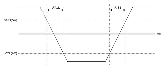
Figure 42 tRISE and tFALL Definition for Output Slew Rate, NV-DDR2/3 (single-ended)
