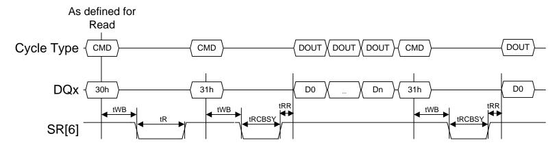
Figure 99 Read Cache Sequential timing, start of cache operations
