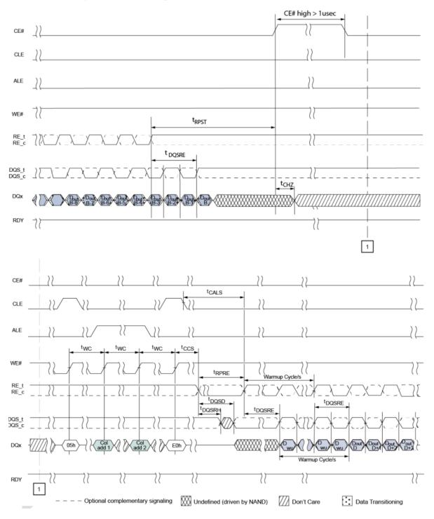
Figure 39 Example of Data Output Pausing for greater than 800 MT/s
