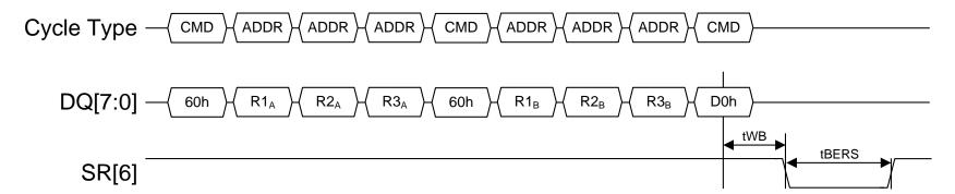
Figure 139 Multi-plane Block Erase timing, ONFI-JEDEC Joint Taskgroup primary definition
