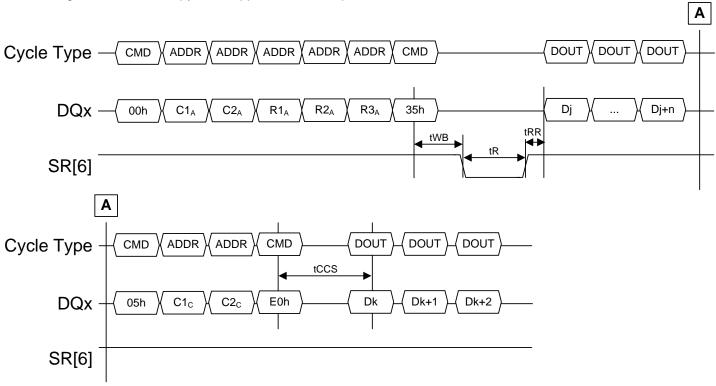
Figure 106 Copyback Read with data output
