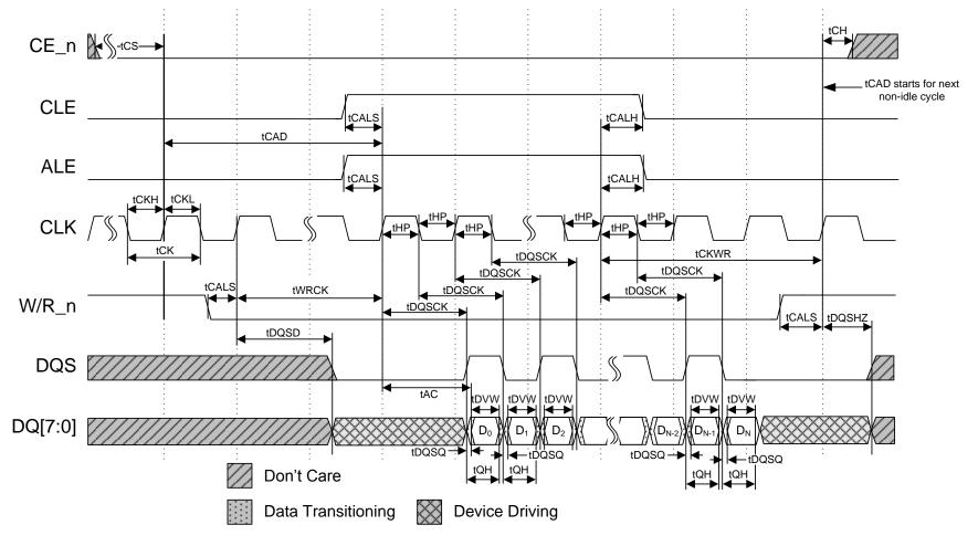
Figure 68 Data output cycle timing
