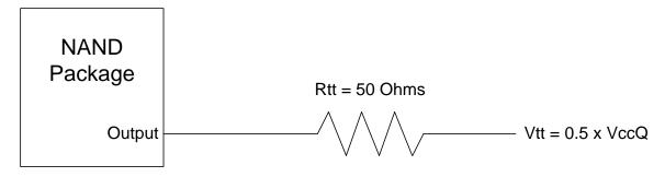
Figure 40 Driver Output Reference Load
