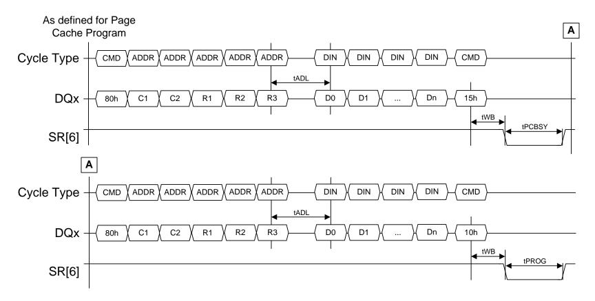
Figure 104 Page Cache Program timing, end of operations
