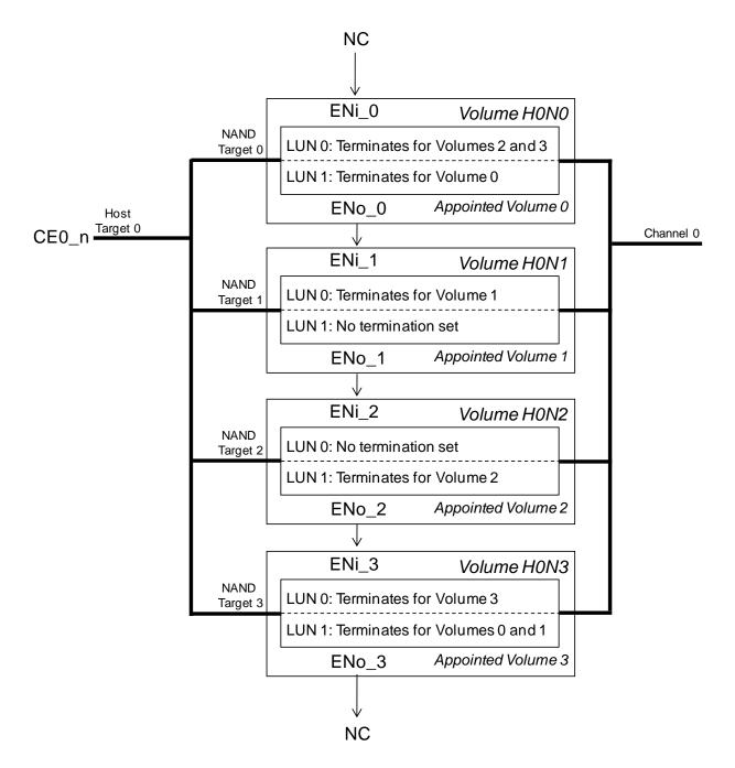
Figure 54 Example: Non-Target ODT for Data Output, Target ODT for Data Input
