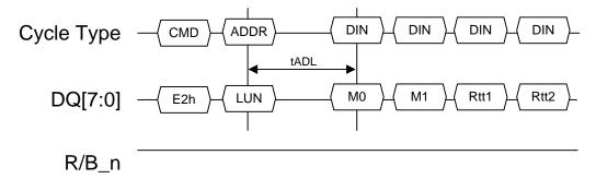
Figure 116 ODT Configure timing diagram
