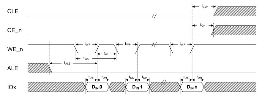
Figure 58 Data input cycle timings
