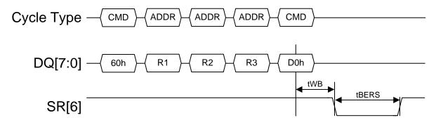
Figure 92 Block Erase timing
