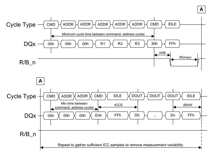
Figure 147 ICC4R and ICCQ4R measurement procedure
