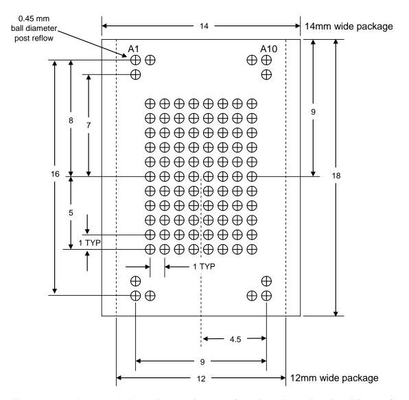
Figure 13 BGA-100 ball spacing requirements (top view, dimensions in millimeters)
