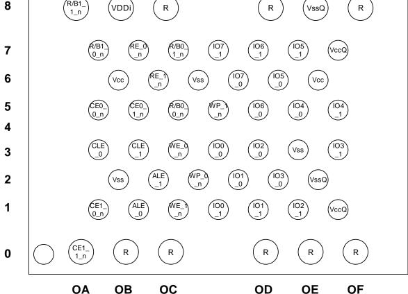
Figure 4 LGA pinout for 8-bit data access
