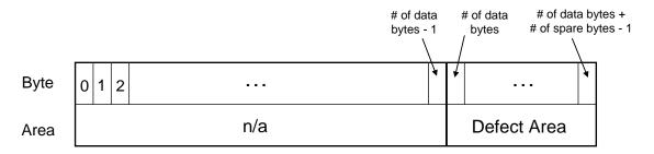
Figure 35 Area marked in factory defect mapping
