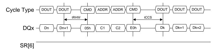
Figure 110 Change Read Column timing
