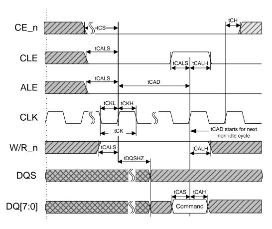
Figure 63 Command cycle timings
