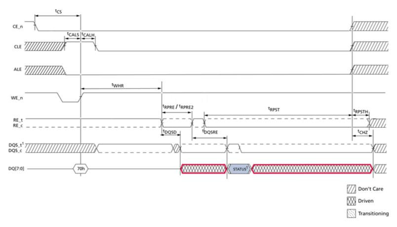
Figure 96 Read Status command using NV-DDR2/3 data interface
