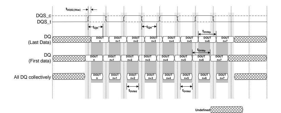
Figure 77 Data output cycle timing (after training)
