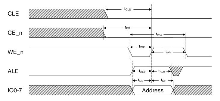
Figure 57 Address latch timings
