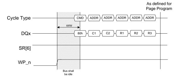
Figure 27 Write Protect timing requirements, example
