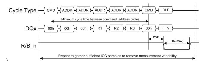
Figure 144 ICC1 measurement procedure
