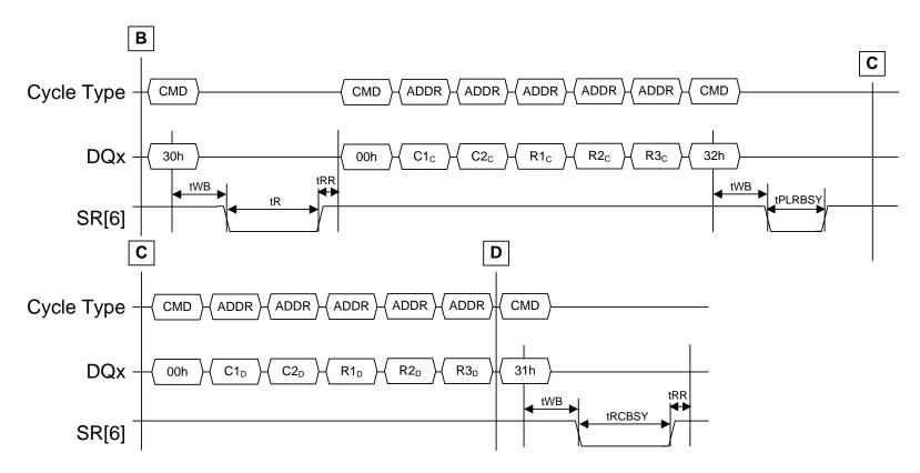
Figure 143 Multi-plane Read Cache Random command issue timing
