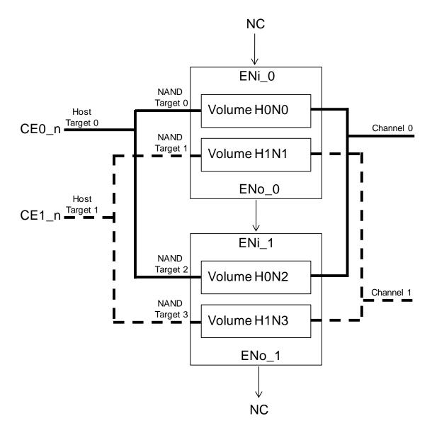
Figure 29 CE\_n Pin Reduction Topology, example 2
