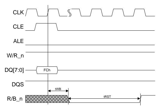
Figure 83 Synchronous Reset timing diagram
