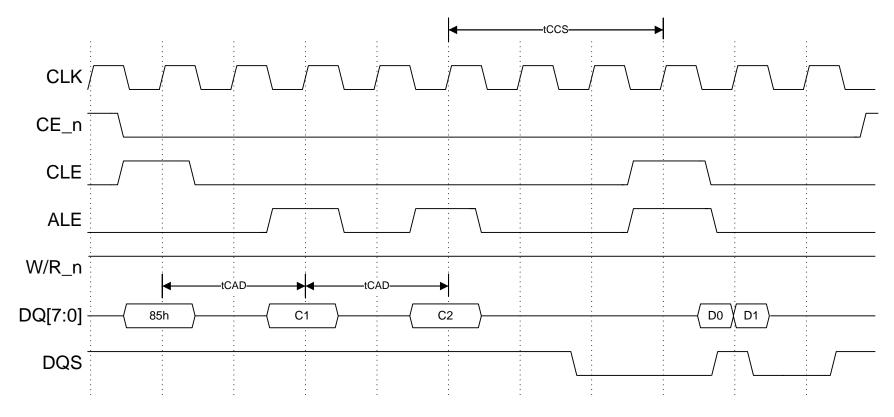
Figure 80 NV-DDR data interface command description
