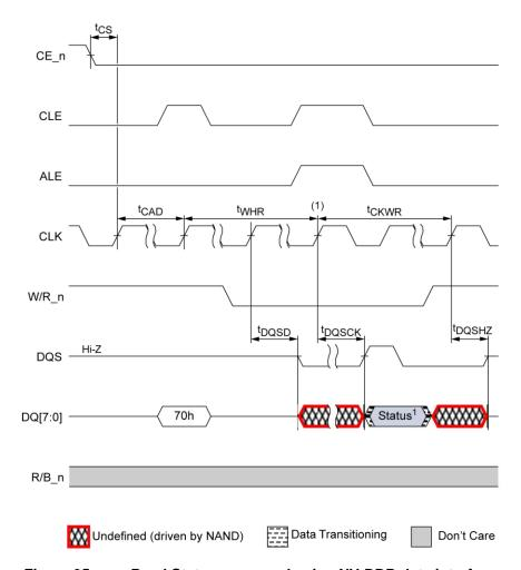
Figure 95 Read Status command using NV-DDR data interface
