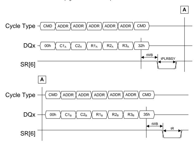
Figure 136 Multi-plane Copyback Read timing for Multi-plane Copyback Program
