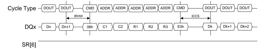
Figure 111 Change Read Column Enhanced timing
