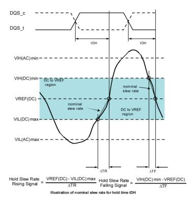
Figure 48 Nominal Slew Rate for Data Hold Time (tDH)
