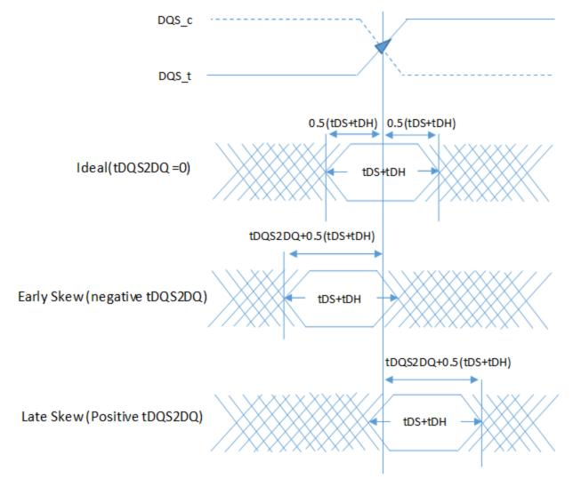
Figure 75 Data input cycle timing (after training)
