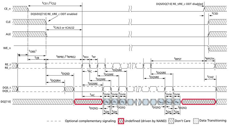
Figure 76 Data output cycle timing (no training on DQ)
