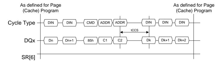
Figure 113 Change Write Column timing
