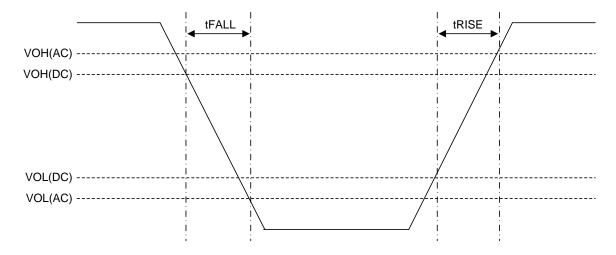
Figure 41 tRISE and tFALL Definition for Output Slew Rate, NV-DDR
