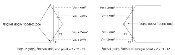
Figure 150 Two point method for measuring timing parameters with tri-state condition
