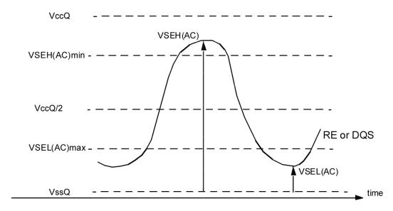
Figure 24 Single-Ended Requirements for Differential Signals
