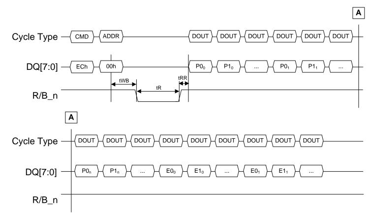
Figure 90 Read Parameter Page command timing
