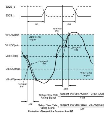
Figure 47 Tangent Line for Data Setup Time (tDS)
