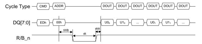
Figure 91 Read Unique ID command timing
