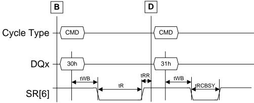
Figure 142 Multi-plane Read Cache Sequential command issue timing
