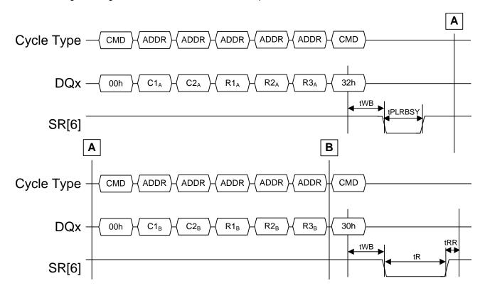
Figure 140 Multi-plane Read command issue timing
