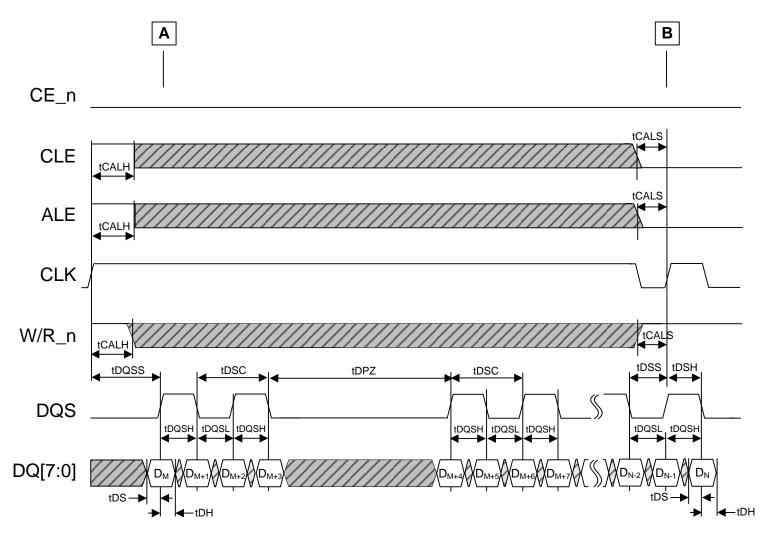
Figure 67 Data input cycle timing, CLK stopped with data pause
