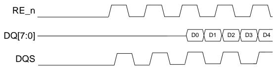
Figure 50 Warmup Cycles for Data Output
