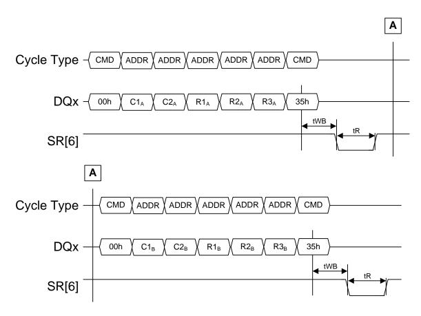
Figure 135 Non-multi-plane Copyback Read timing for multi-plane Copyback Program
