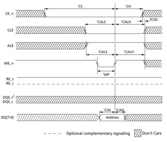
Figure 73 Address cycle timings
