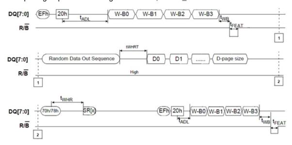
Figure 124 DCC (RE t/c) Training using Set Feature
