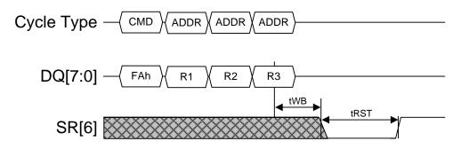
Figure 84 Reset LUN timing diagram
