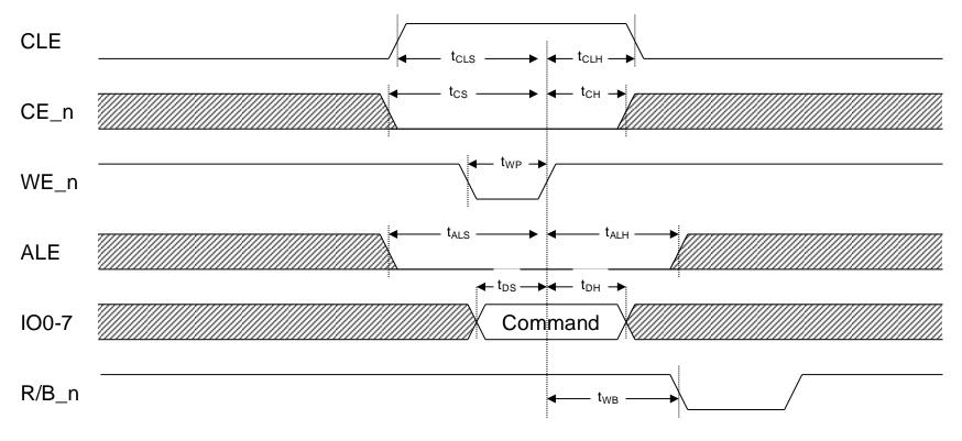
Figure 56 Command latch timings
