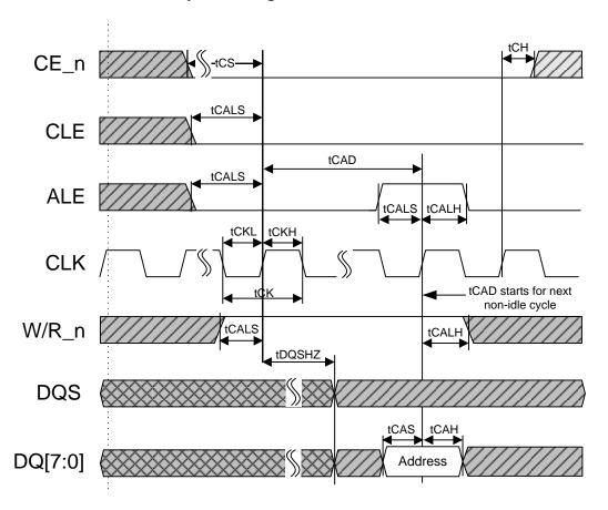
Figure 64 Address cycle timings
