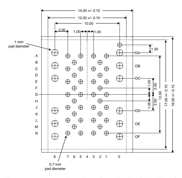
Figure 6 LGA-52 pad spacing requirements (bottom view, dimensions in millimeters)
