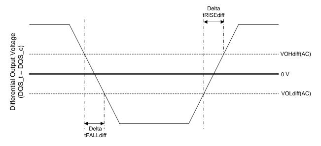
Figure 43 tRISEdiff and tFALLdiff Definition for Output Slew Rate, NV-DDR2/3 (differential)
