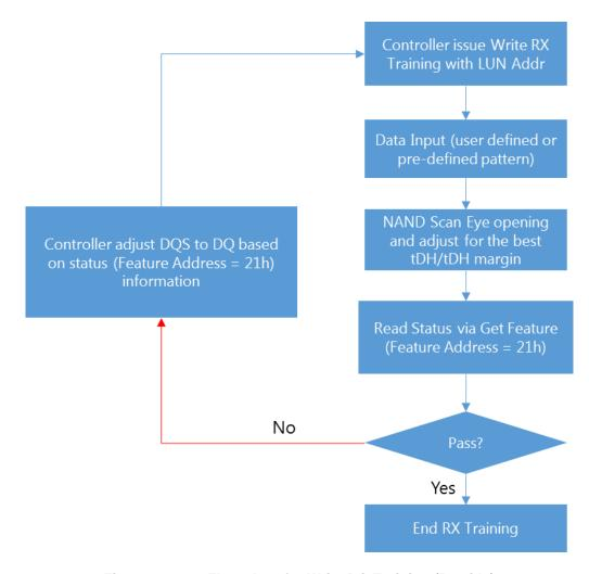
Figure 130 Flow chart for Write DQ Training (Rx side)
