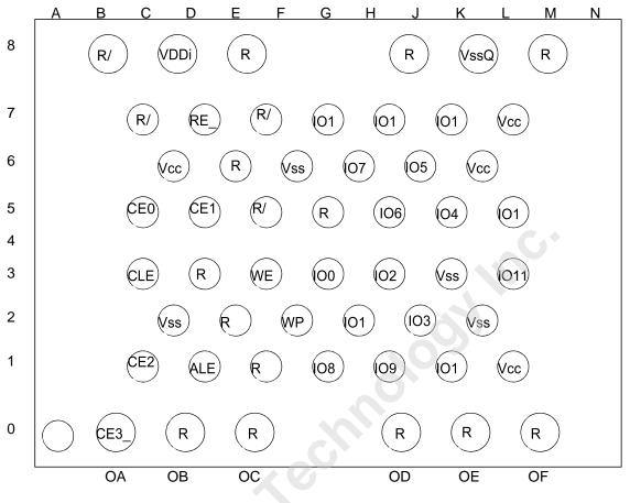
Figure 10 — LGA pinout for 16-bit data access
