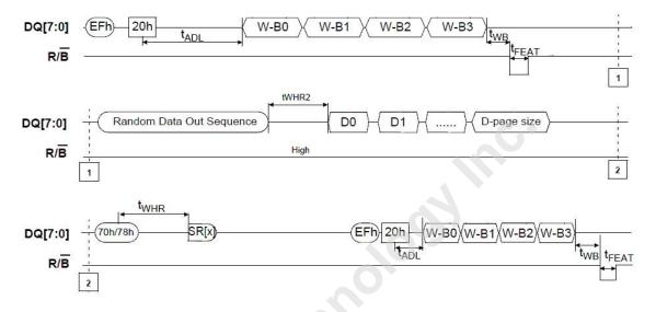
Figure 28 — DCC (RE\_t/c) Training using Set Feature
