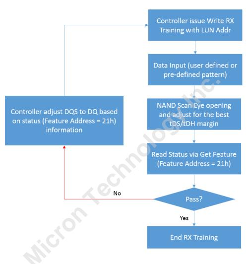
Figure 34 — Flow Chart for Write DQ Training (Rx side)
