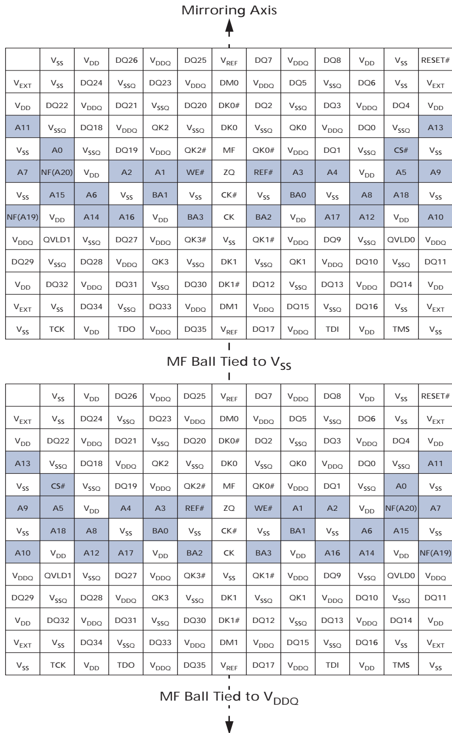
Figure 3: Ball Assignments with Mirror Function in Opposite States
