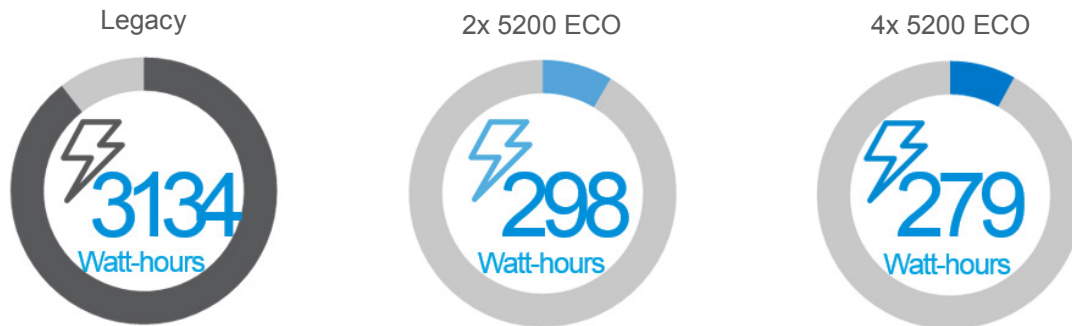
Figure 2b: Energy Consumed to Complete Query Set by Configuration (Stream Count = 8; Scale Different from Figure 2a)
