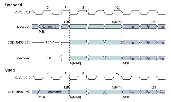
Notes: 1. For extended SPI protocol,  $C_x = 7 + (A[MAX] + 1)/4$ ; For quad SPI protocol,  $C_x = 1 + (A[MAX] + 1)/4$ .
