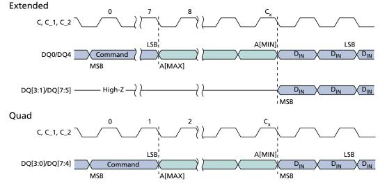
Notes: 1. For extended SPI protocol,  $C_x = 7 + (A[MAX] + 1)$ ; For quad SPI protocol,  $C_x = 1 + (A[MAX] + 1)/4$ .
