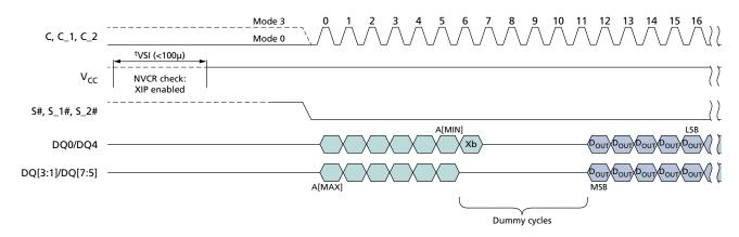
Note: 1. Xb is the XIP confirmation bit and should be set as follows: 0 to keep XIP state; 1 to exit XIP mode and return to standard read mode.
