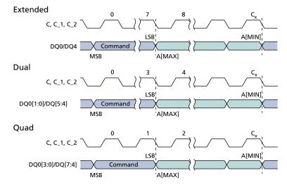
Notes: 1. For extended SPI protocol,  $C_x = 7 + (A[MAX] + 1)$ ; For dual SPI protocol,  $C_x = 3 + (A[MAX] + 1)/2$ ; For quad SPI protocol,  $C_x = 1 + (A[MAX] + 1)/4$ .
