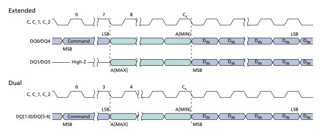
Notes: 1. For extended SPI protocol,  $C_x = 7 + (A[MAX] + 1)/2$ ; For dual SPI protocol,  $C_x = 3 + (A[MAX] + 1)/2$ .
