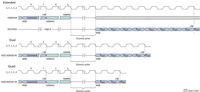
Notes: 1. For extended protocol,  $C_x = 7 + (A[MAX] + 1)$ ; For dual protocol,  $C_x = 3 + (A[MAX] + 1)/2$ ; For quad protocol,  $C_x = 1 + (A[MAX] + 1)/4$ .
