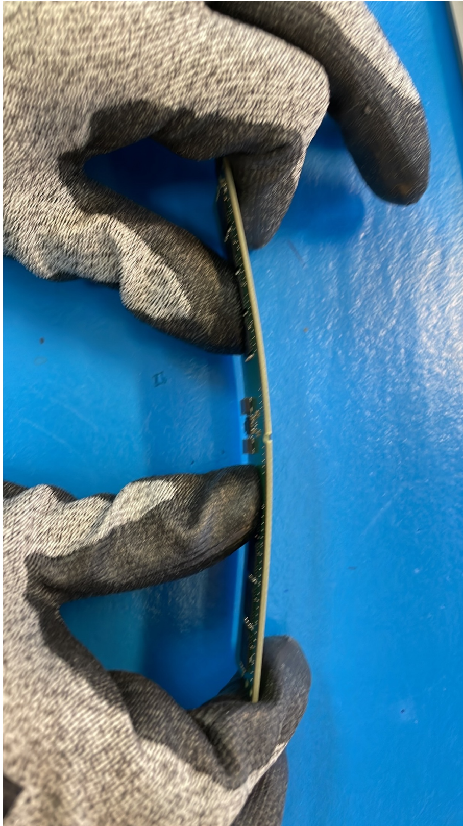
Figure 16: Never Bend or Twist a Board-Level Product
