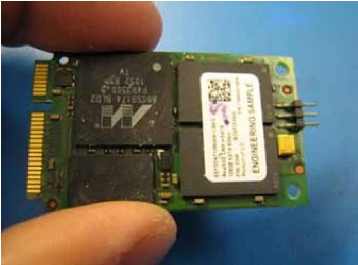
Figure 8: Proper Way to Hold an mSATA is by the Edges
