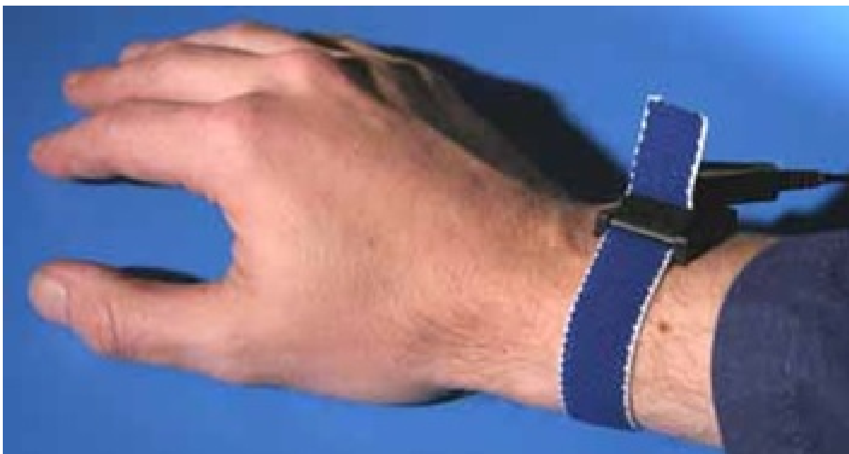
Figure 6: Always Wear ESD Straps When Handling, Inserting, or Removing Modules and SSDs into Sockets
