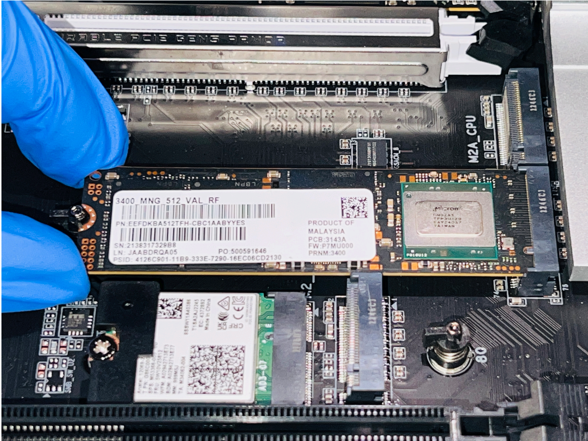
Figure 43: Hold the PCB Against Standoff after Insertion
