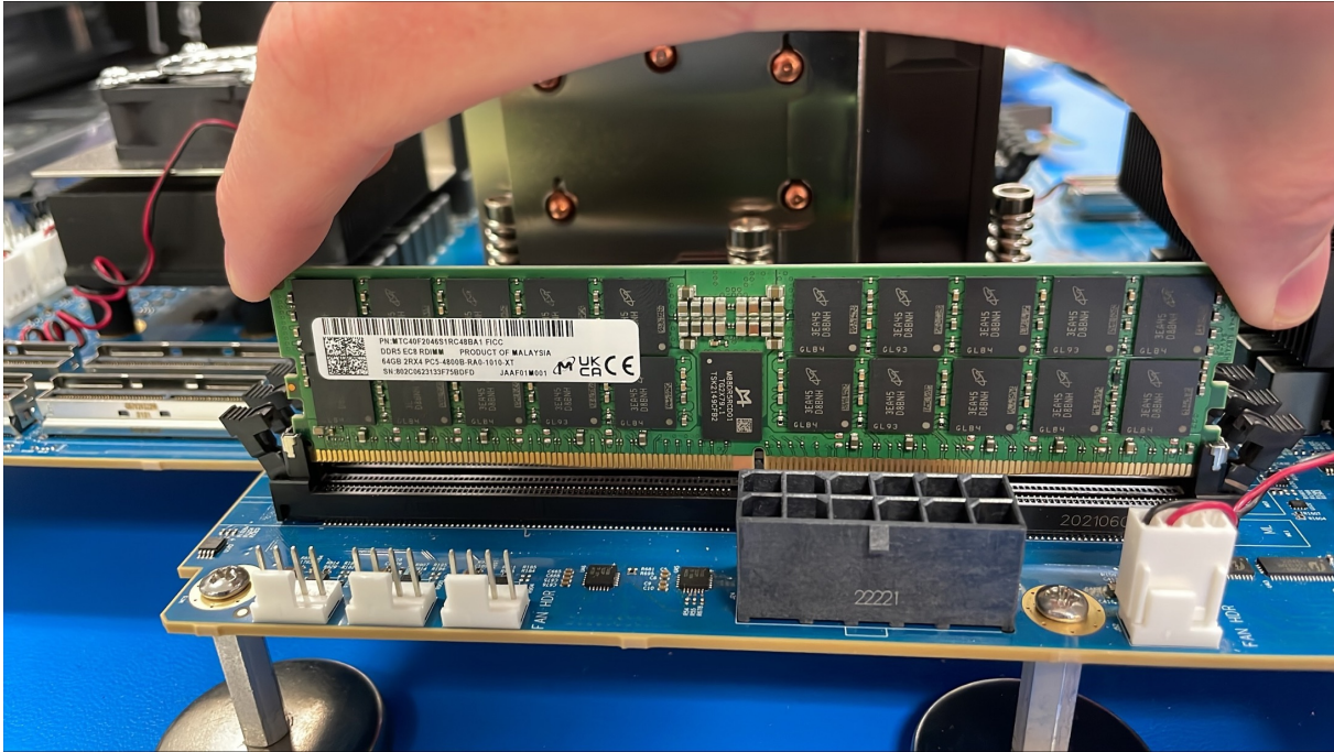
Figure 51: Remove the DIMM, Touching Only the Edges of the PCB
