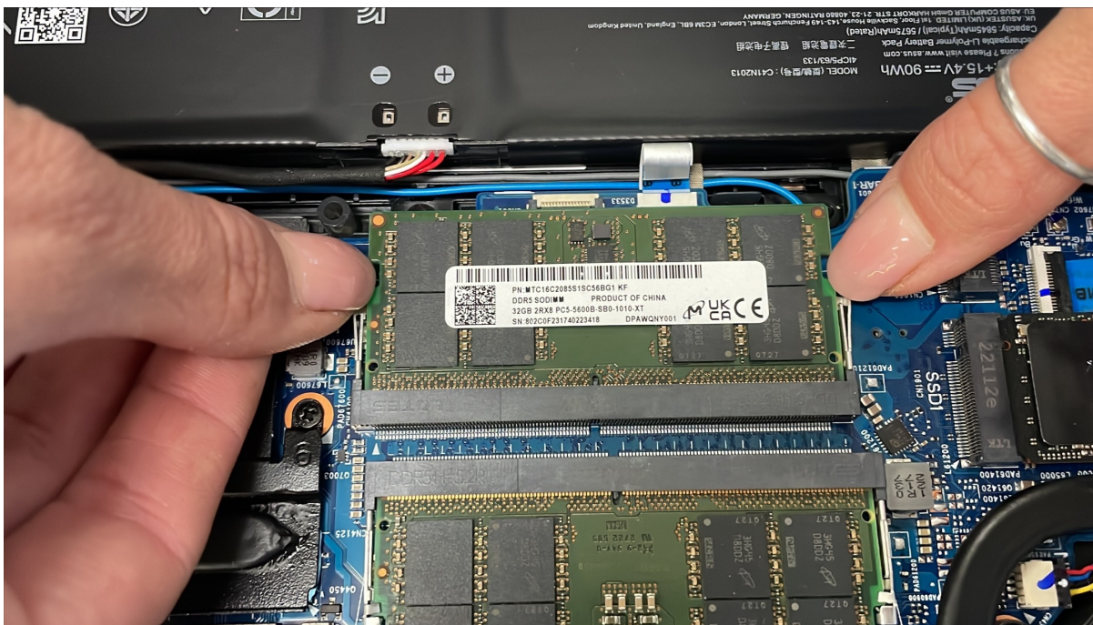
Figure 46: Release the Clips on the Sides of the Socket
