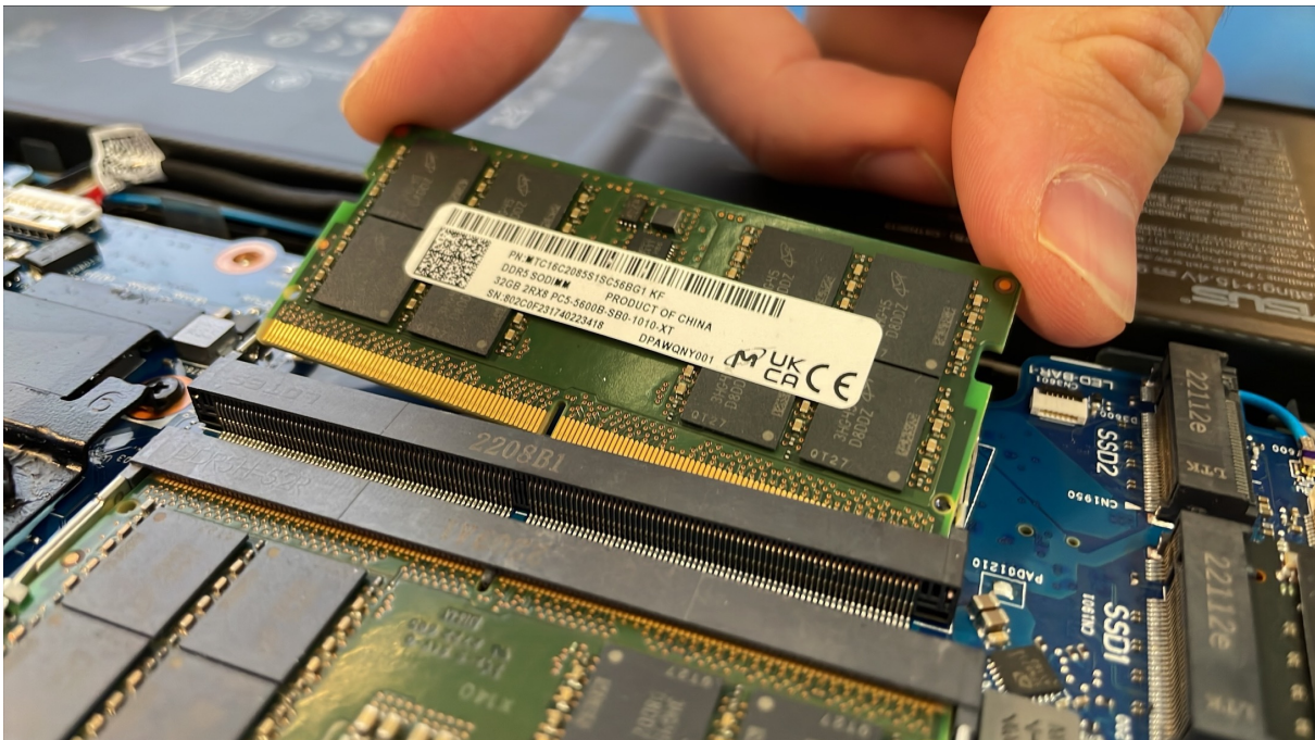
Figure 25: Never Insert Modules at an Angle and Never Insert One Side at a Time
