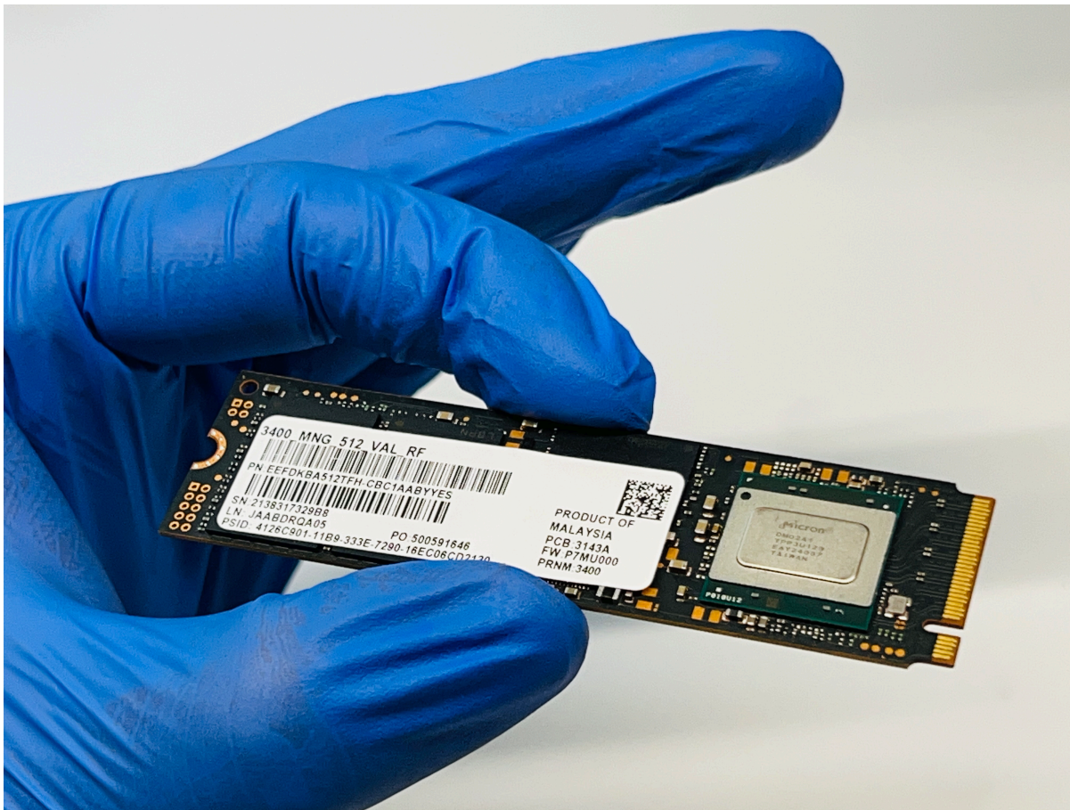
Figure 10: Proper Way to Hold an M.2 SSD is by the Sides
