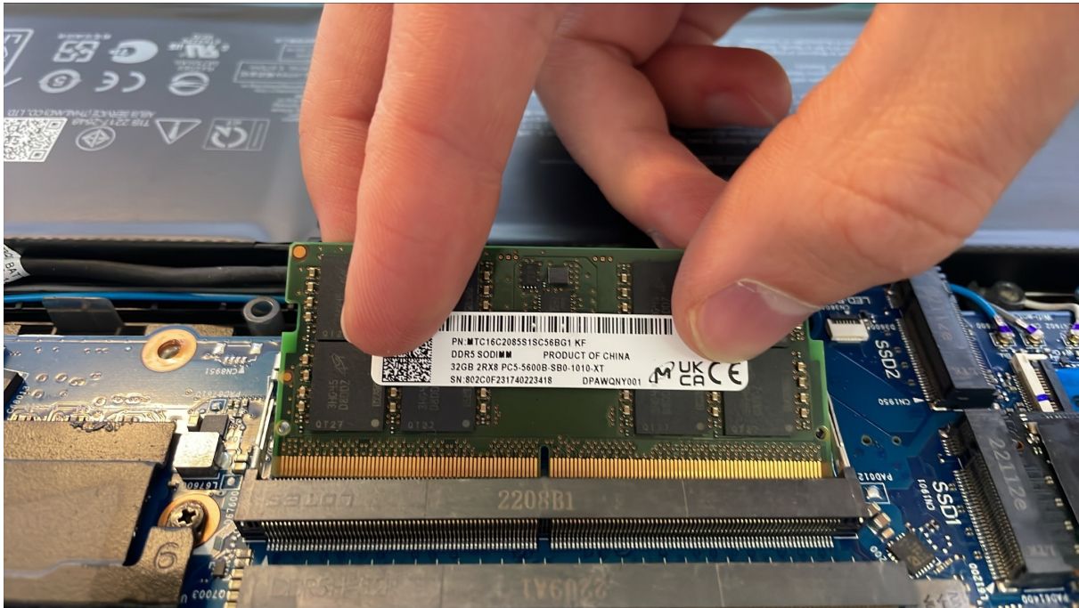
Figure 54: Never Remove the Module at an Angle
