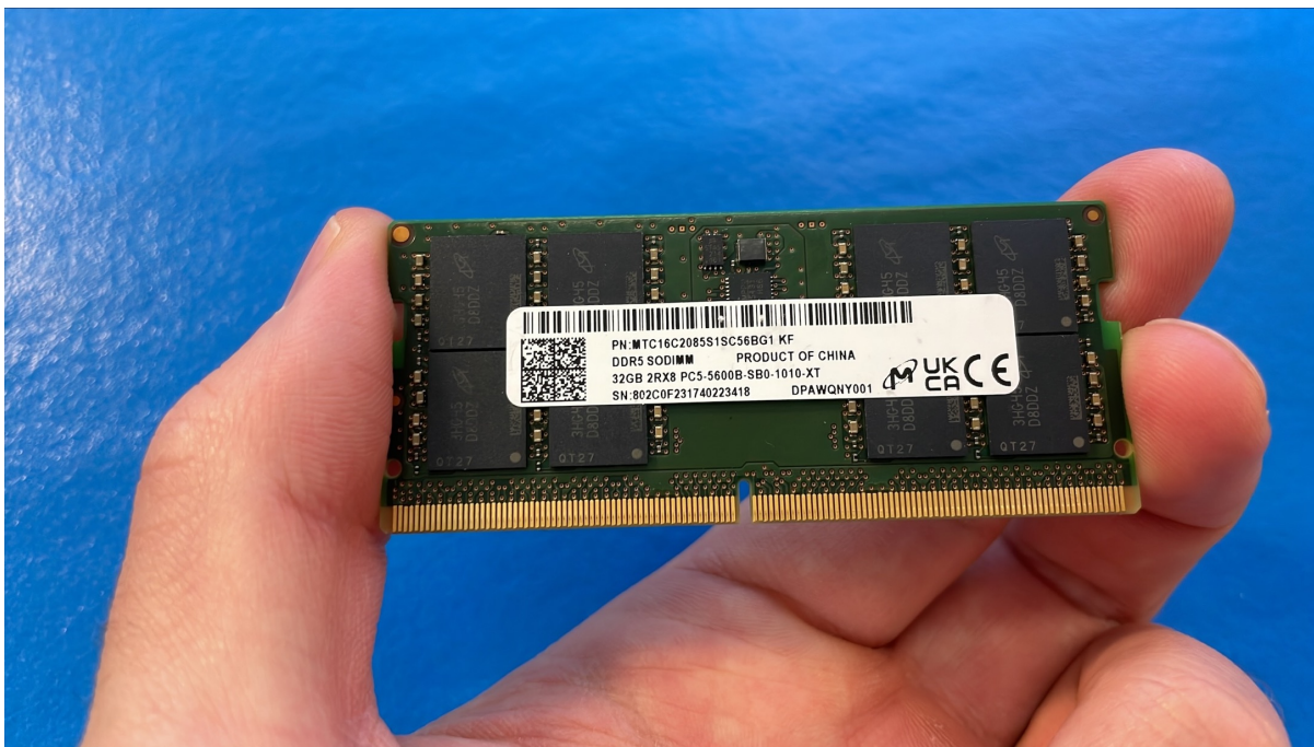
Figure 7: Proper Way to Hold a Module is by the Edges
