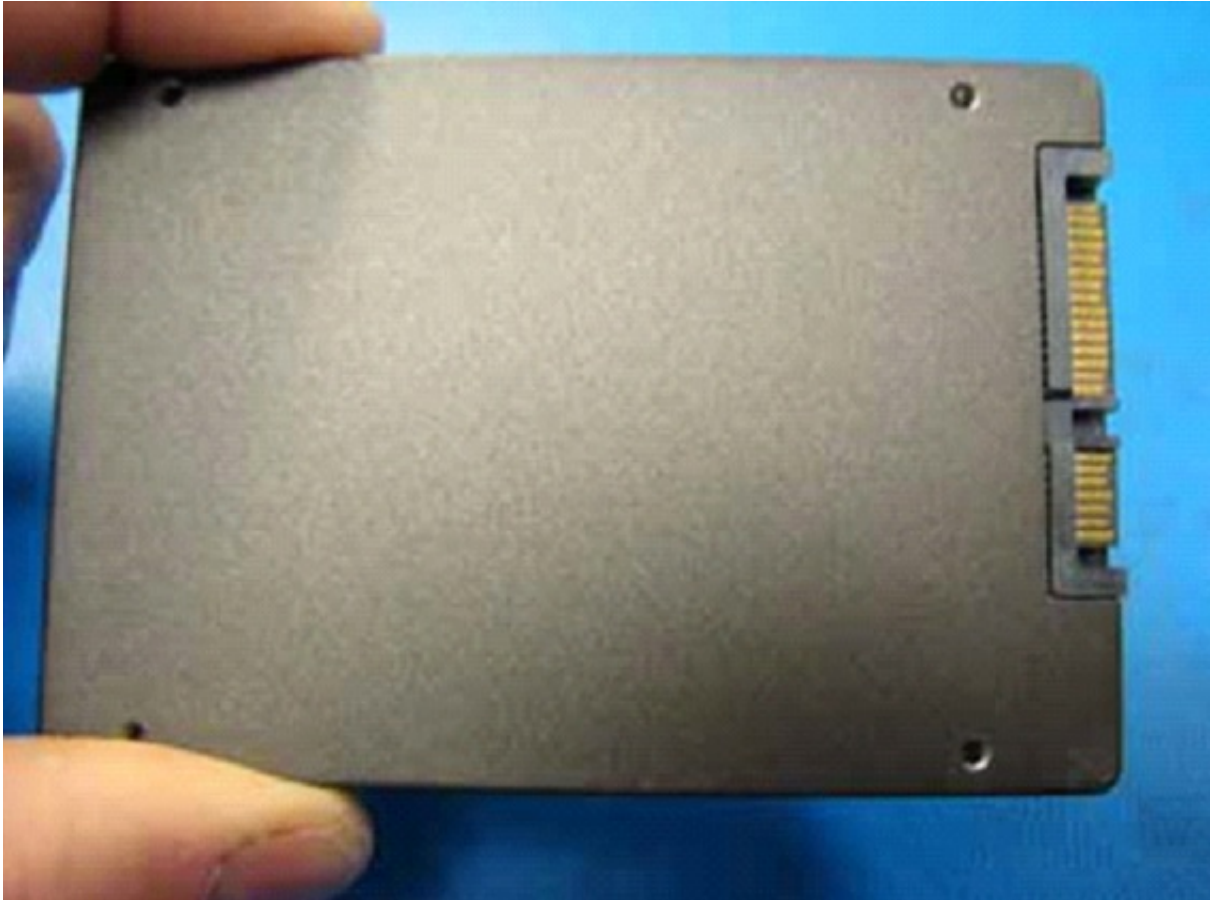
Figure 9: Proper Way to Hold an SSD is by the Sides
