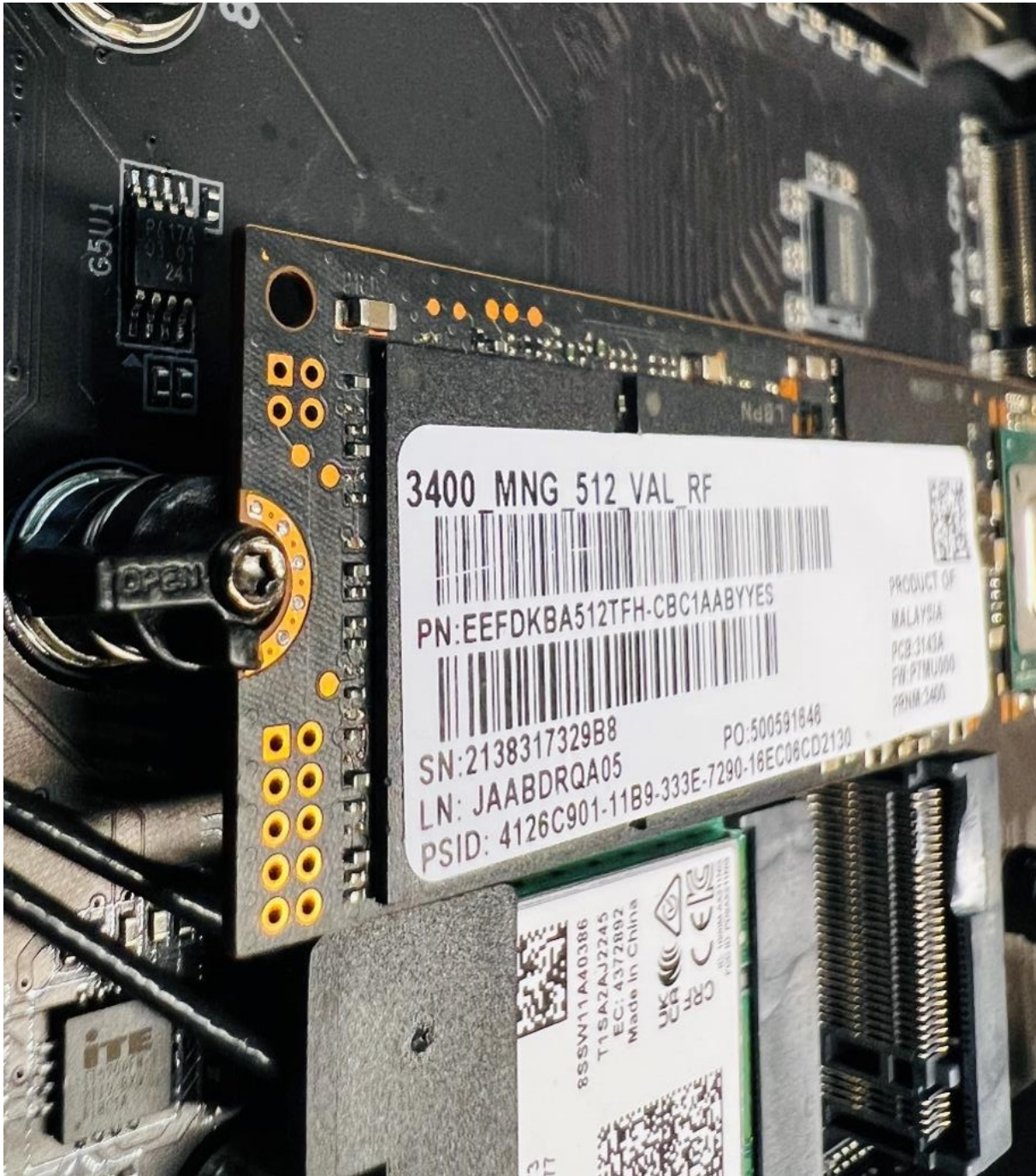
Figure 44: Screw Insertion and Tightening to Complete Installation
