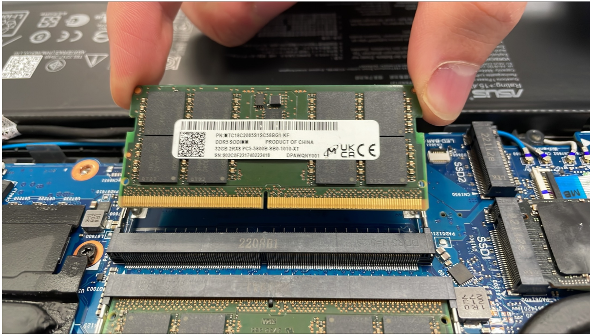
Figure 47: Remove the Module, Touching Only the Edges of the PCB
