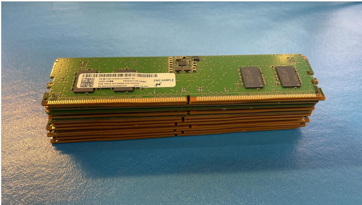
Figure 18: Never Stack Two or More Board-Level Products
