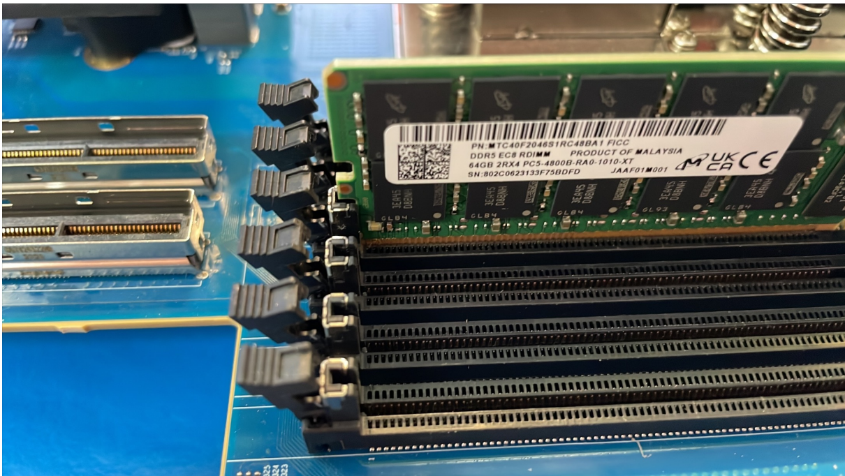
Figure 31: Step 3a – Check the Alignment of the Module and the Ejector Pins/Latches
