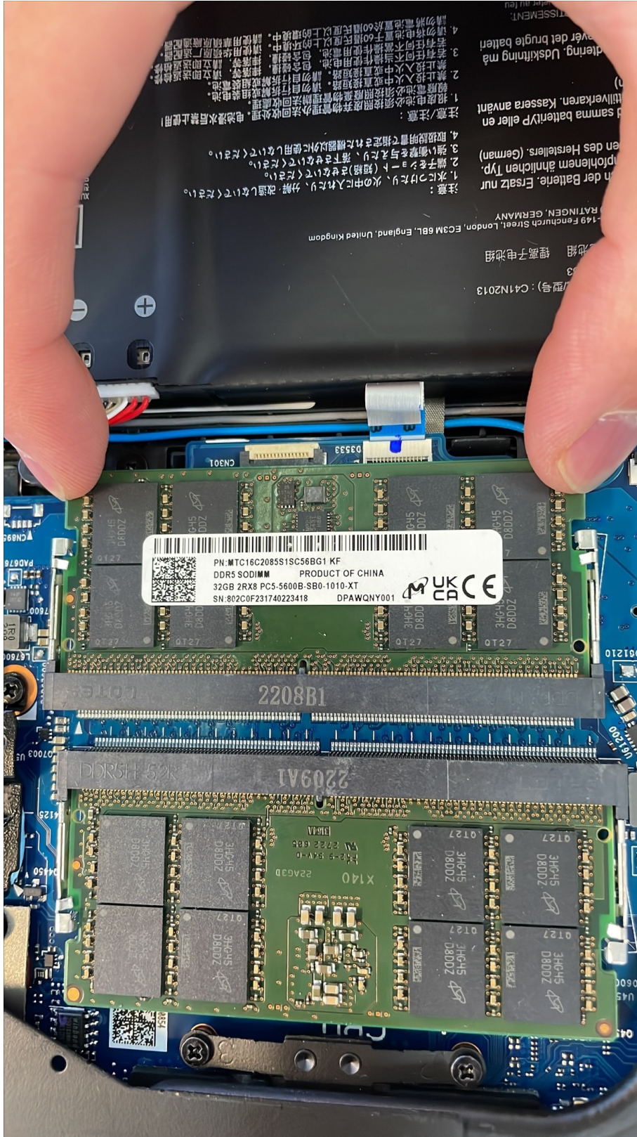
Figure 22: Step3 – Press Down on the PCB to Set the Module into Its Final Position
