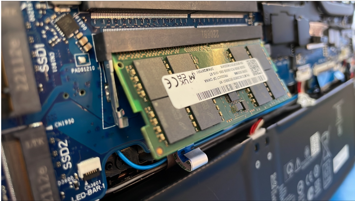
Figure 21: Step2b – Visually Inspect the Angle of Insertion
