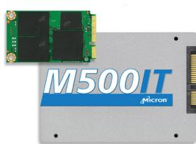
Newer drives like the M500IT have transitioned to lead-free BGA-based packages, which provide a greater strength-to-weight ratio in terms of their mechanical adherence to the PCB.
